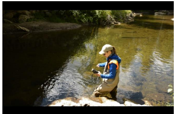
5 / 6 Nottawasaga Valley Conservation Authority staff measure water quality with a multiparameter sonde. It measures parameters that would change by the time a water sample got to a lab. Photo supplied by the Nottawasaga Valley Conservation Authority
