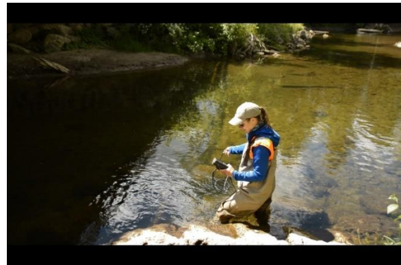
5 / 6 Nottawasaga Valley Conservation Authority staff measure water quality with a multiparameter sonde. It
