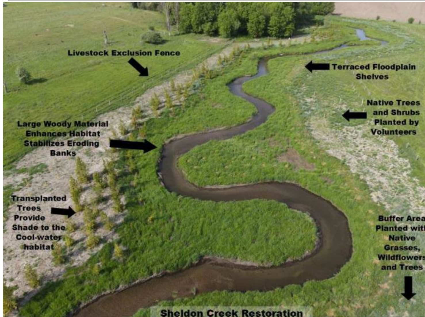
Figure 3: Overview of a typical river restoration project focused on increasing flood storage, reducing/mitigating erosion potential of the river, and improving riparian and aquatic habitat.
